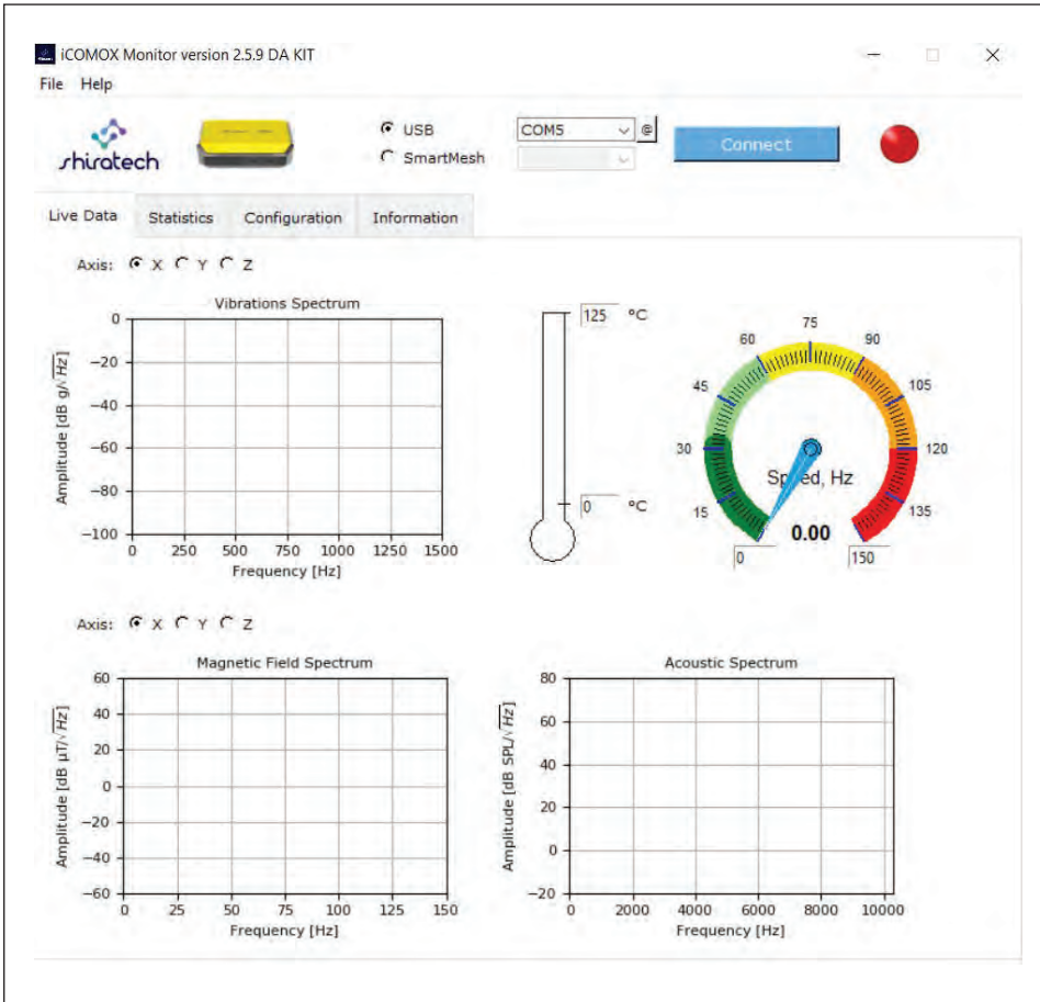
Figure 16: The iCOMOX interface (Image: EE Times Europe)
