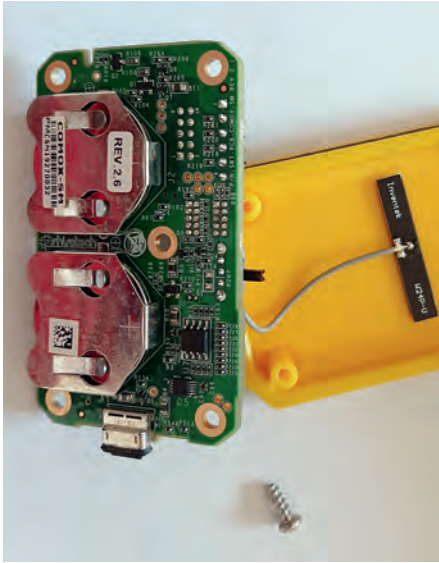
Figure 11: The coin-cell batteries powering the board (Image: EE Times Europe)
