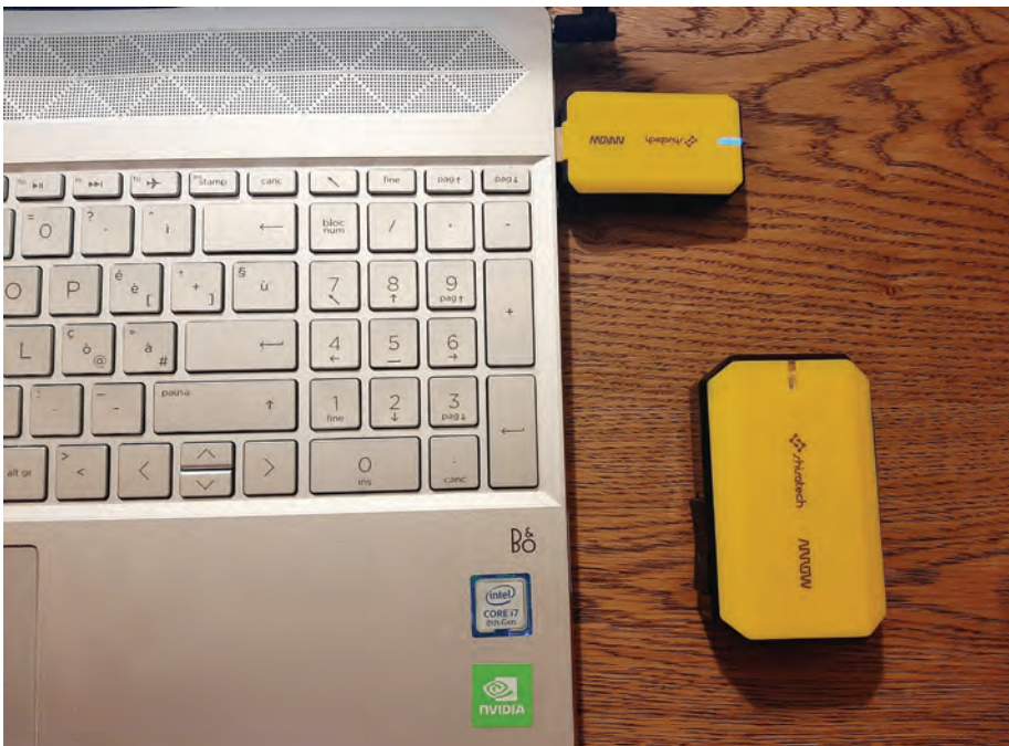
Figure 15: The dongle connected to the USB port for SmartMesh communication with the board (Image: EE Times Europe)
