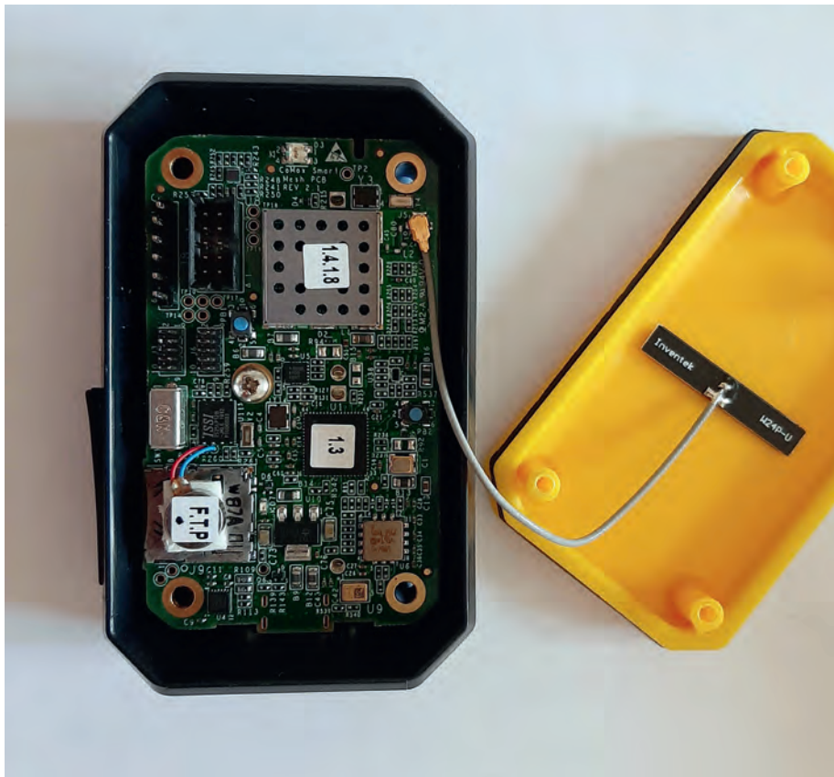
Figure 10: Inside of the board with electronics on the left and SmartMesh antenna on the right (Image: EE Times Europe)
