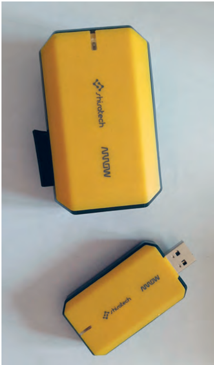
Figure 4: The card (top) and the wireless hub for SmartMesh control (Image: EE Times Europe)
